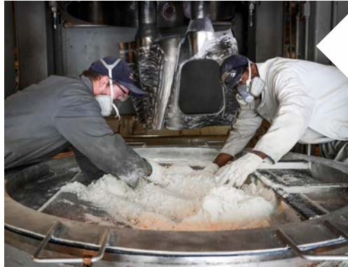
Naval Surface Warfare Center Indian Head Explosive Ordnance Disposal Technology Division Energetics Manufacturing Department's Explosives and Energetics Division operators screen energetic material at the command's 420 gallon mixer. (U.S. Navy photo by Matthew Poynor/RELEASED)
